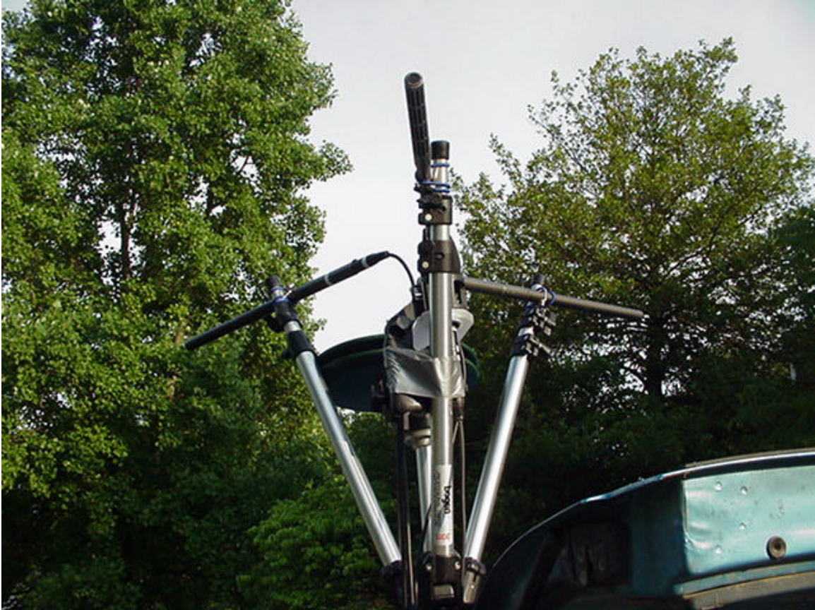
Figure 3. The antenna array used to capture ambient sounds during BBS surveys. See Table 2 for description of microphones. Most important are the three long, thin directional microphones pointing away from the center with an angular separation of 120 degrees. Because such microphones drop off in sensitivity away from their axis of orientation, the three channels recorded from these microphones emphasized different sections of the soundscape, facilitating localization of the sound sources during post-processing of recordings.
